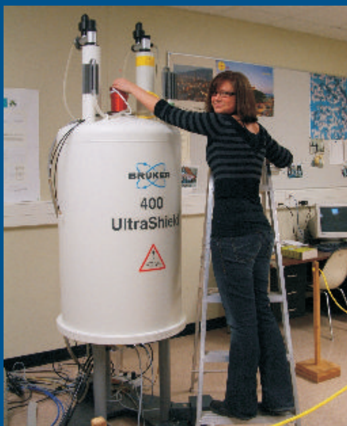
Chemistry student Clare McConkey inserts her sample into the 400MHz Nuclear Magnetic Resonance Spectrometer for analysis.
